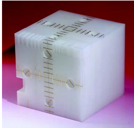
The CT Simulation Phantom tests all quality control parameters that can affect patient treatment, including RRE, magnification, image quality, and more
