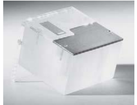
Phantom with two 5-20 LP/mm test patterns (optional) in parallel and perpendicular orientation. Also includes an air step wedge with aluminum attenuator
